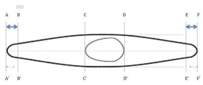
Section AA' to BB' - Front Impact Zone - measured to the point 100mm down the length of the kayak 100 mm minimum radius at any point on B-A-B'
